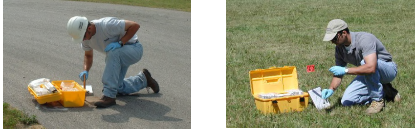
Figure 3 — Installation of Samplers with Beacon Environmental’s BESURE Kit™
