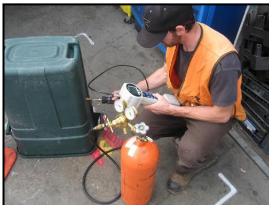
Monitoring leak check compound within shroud during sample collection
