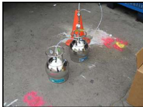
Sample collection with Summa canisters
