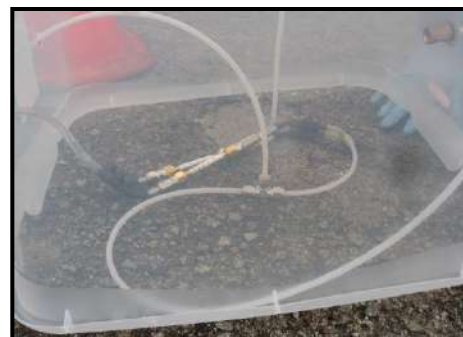
Sample collection with sorbent tube
