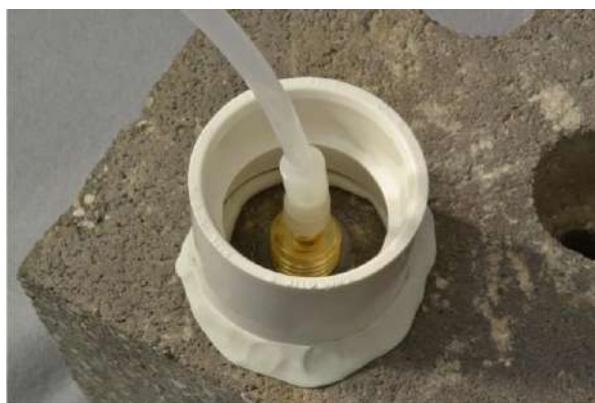
Figure 6. Water dam used for leak detection
